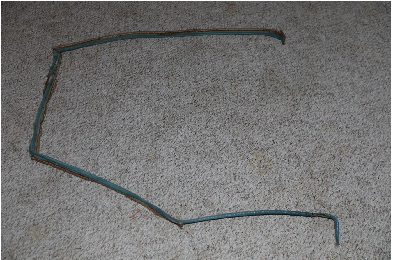
The original removed from passenger front door opening. Hard, dry, shriveled and crumbly.
