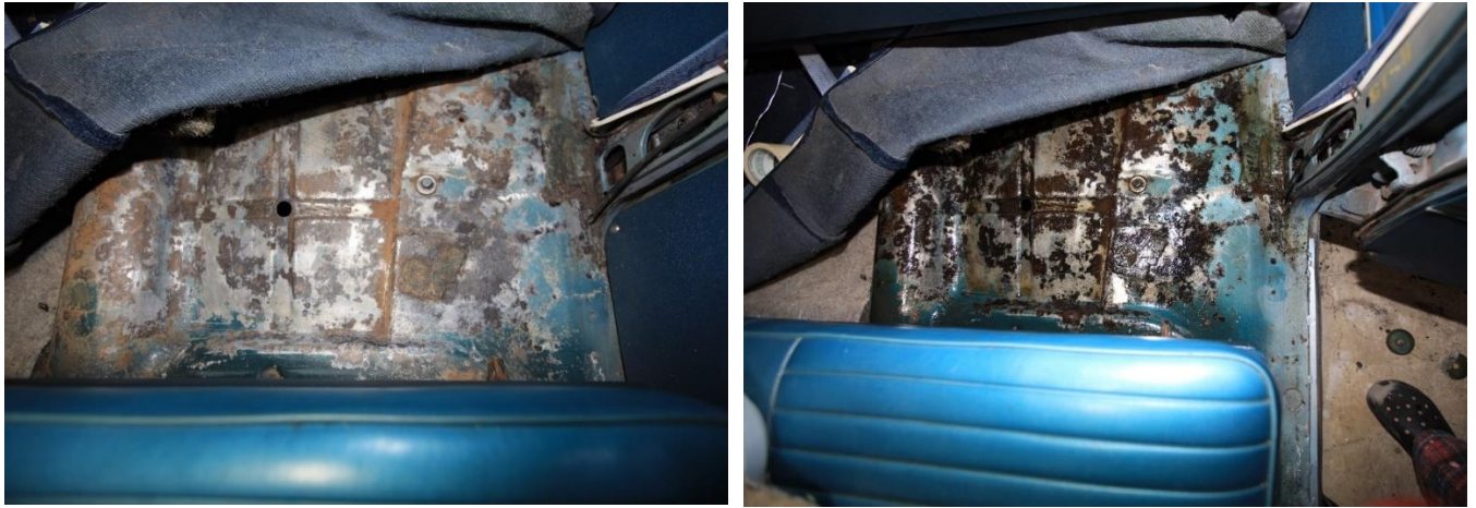
Treated with phosphoric acid, sanded with #80 sandpaper, and treated with clear POR-15
