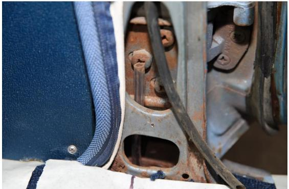
Passenger-side front sliding roof drain tube. Note the rust where water had been draining. Treated with phosphoric acid and followed by a generous coating of POR-15 and then a color coat.
