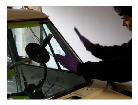
Adam then shot a bead of the bedding compound under the windshield side of the gasket...
