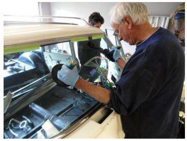
Adam pulled the rope and the lip of the gasket fell neatly into place...
