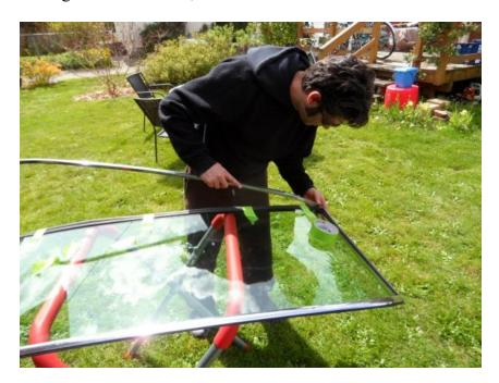
...and taped the gasket to the window in several spots to insure it stayed in place...
