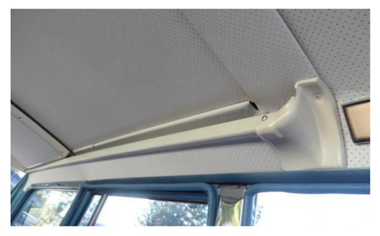
The crossbar that covers the joint between the front and middle panels was covered in the same headliner material and installed...
