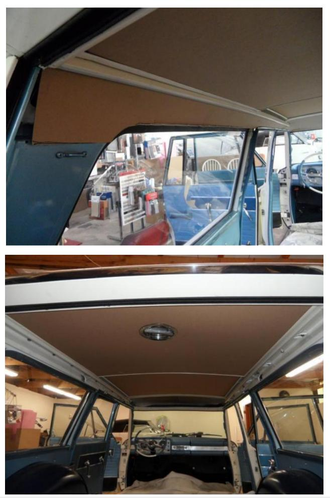
He used a heavy coated and embossed panelboard from <u>PerfectFit</u> which is his wholesale supplier. This is also known as Package Tray Panel Board. The material is raw cardboard on one side and embossed and coated on the other with a black, vinyl pattern. The coated side will be installed UP and the uncoated side will have the vinyl headliner material glued to it.
