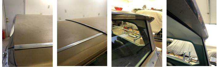
With a fixed roof the tailgate glass no longer needs the chrome frame around only the glass. It now is fully contained in the window channel of the side and top of the window opening.
