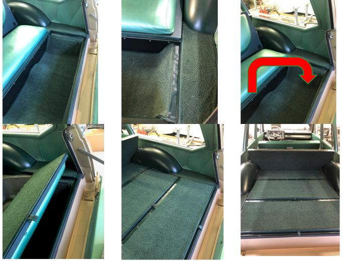
The side panels behind the second row seat, shown above, are the original materials but they were removed and freshened up a little to be compatible with the look of rest of the interior. All of the carpet in the Wagonaire has been replaced using the original as a pattern.
