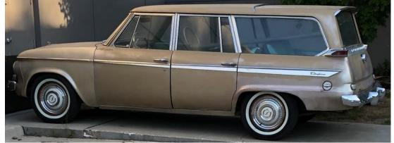
He did his best to match the original color of the roof. He even mixed his own clear coat in order to get the same sheen on the lower body as was evident on the faded roof. The hood and the tailgate were painted separately. The paint on the lower door jambs was spotted in as need from rust repairs but the rest of the jambs looked good and were left original. Dave calls this a "quickie" job but it looks professional to me.
