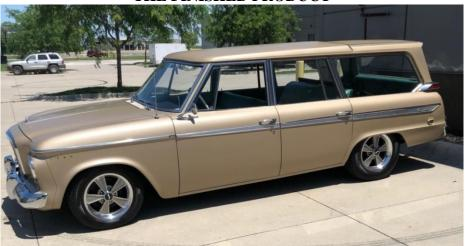
All of the chrome and stainless on the car is original with the exception of the bumpers. Dave secured two NOS 1964 Wagonaire bumpers and bumper guards and installed them on the car.
